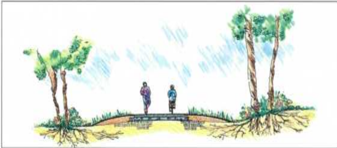
Figure 8 - Above grade cross section is a minimization technique used to protect critical root zones.
