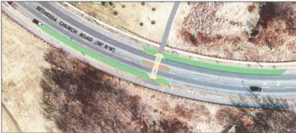
Figure 2 - Proposed at-grade mid-block crossing of Bethesda Church Road with curb bump-outs and a median refuge island. The curb bump-outs will extend for 250 feet in both directions to ensure parked cars can not encroach on sight distance.
