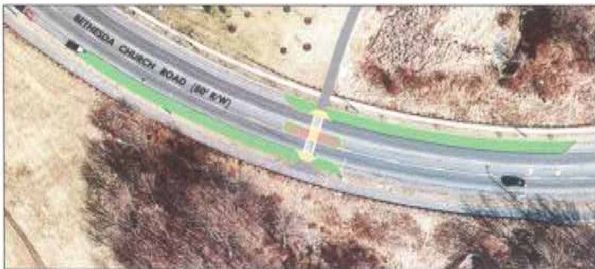
Figure 20 - Proposed at-grade mid-block crossing of Bethesda Church Road with curb bump-outs and a median refuge island.
