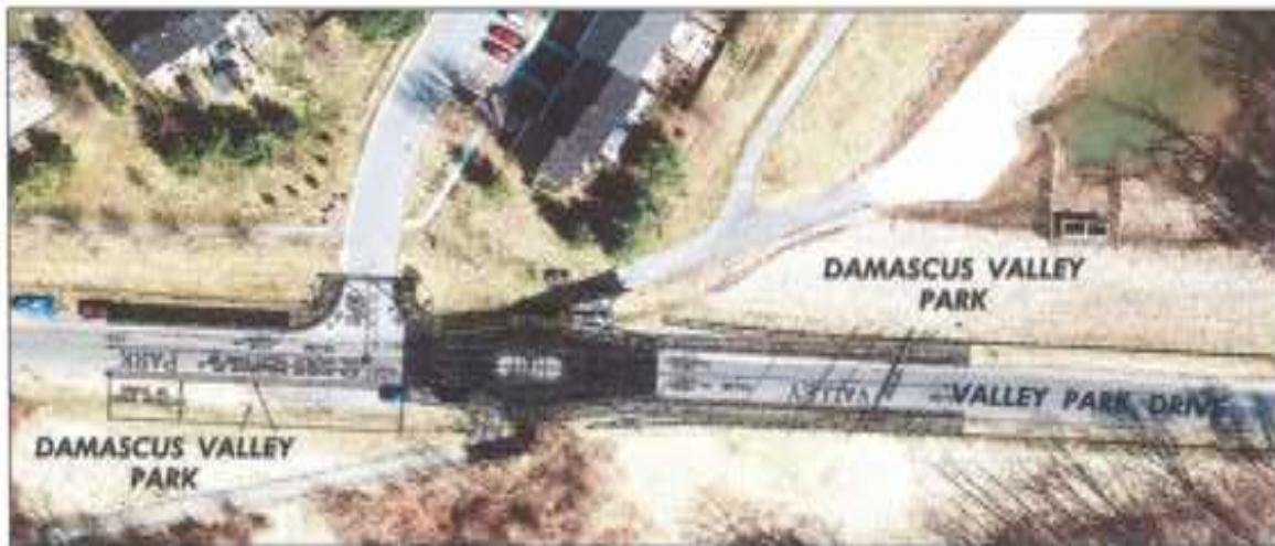
Figure 1 - A roadway crossing at Valley Park Drive is currently under construction by DPW &T with a proposed refuge island for safety. This view shows the design superimposed on an aerial photo of the vicinity.
