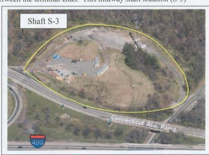
construction process. Almost all tunneled materials will be removed from here and the vast majority of pipe materials will be inserted at this location.
