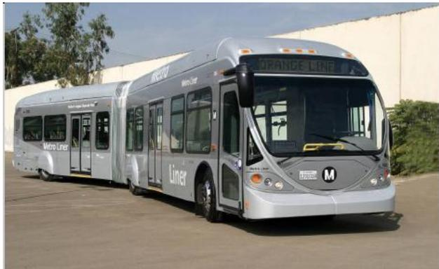
A BRT vehicle can generally accommodate up to 120 passengers (including standees and assuming an articulated bus about 60 feet long as shown left) and can be powered by hybrid-electric, diesel, or compressed natural gas (CNG) engines. The vehicle shown is in use in Los Angeles.
