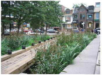
Provide stormwater bio -infiltration areas
