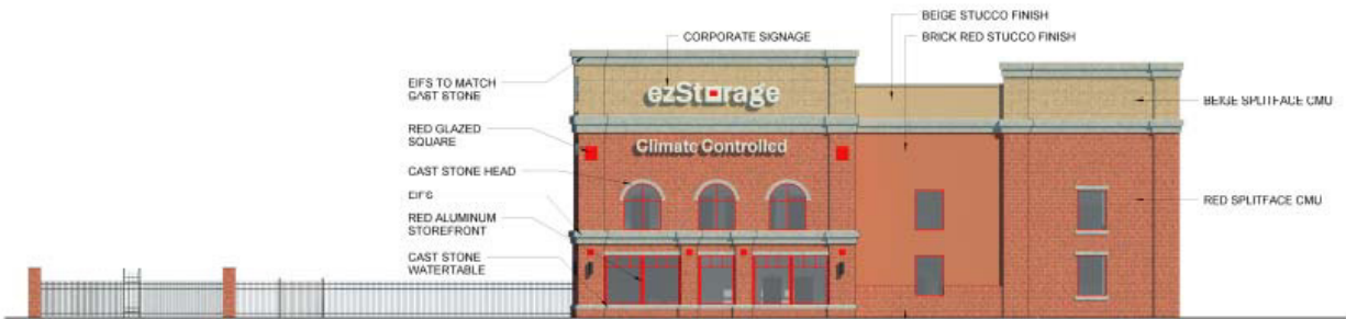
North building elevation
