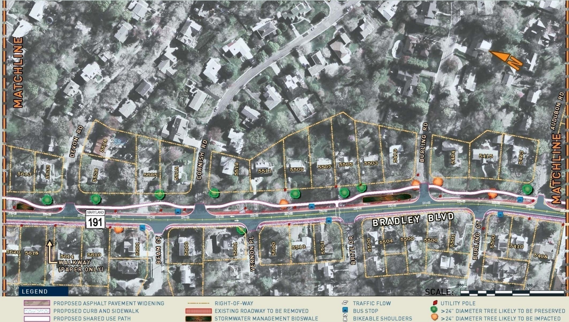
Figure II-18: Alternate 4A – 8' Shared Use Path North Side and Sidewalk South Side with Bikeable Shoulders (RECOMMENDED ALTERNATE)
