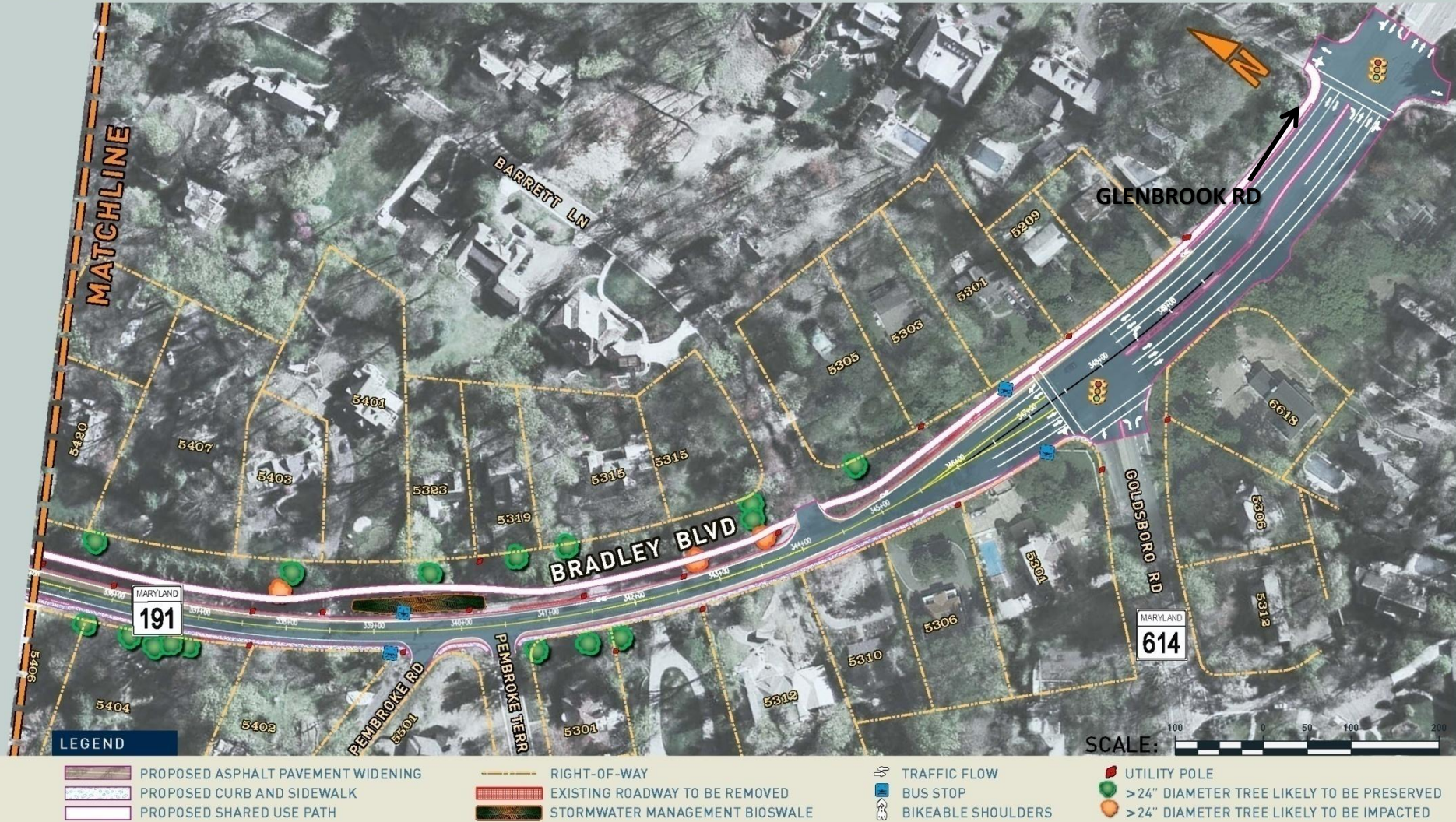
Figure II-19: Alternate 4A – 8' Shared Use Path North Side and Sidewalk South Side with Bikeable Shoulders (RECOMMENDED ALTERNATE)
