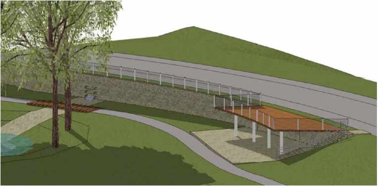
The retaining wall and roof deck shield picnic activities from noise from the road.
