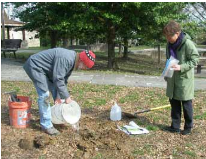
^ Field Percolation Test 1
