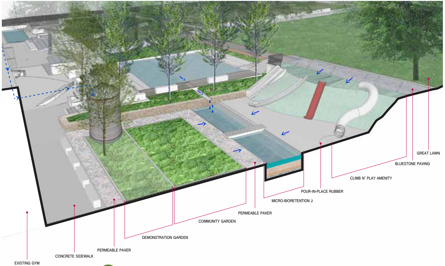
B Cross Section of Bioretention System (North to South at full capacity)
