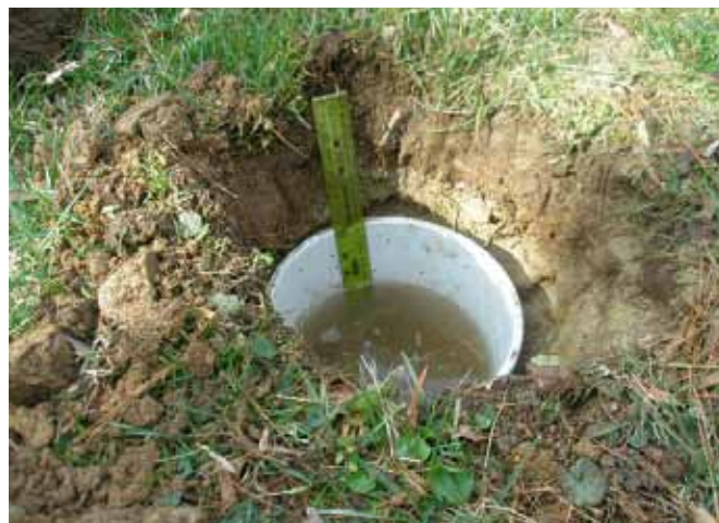
^ Field Percolation Test 2
