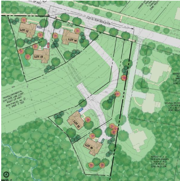
Proposal to have a new driveway within the property boundaries serving Lots 15 and 16.
