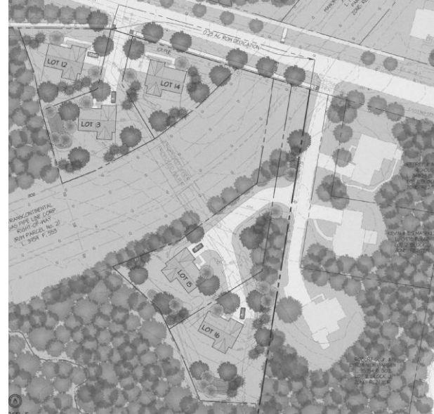
Option to use an existing shared driveway on adjacent property to the east, subject to mutual agreement between all affected property owners.
