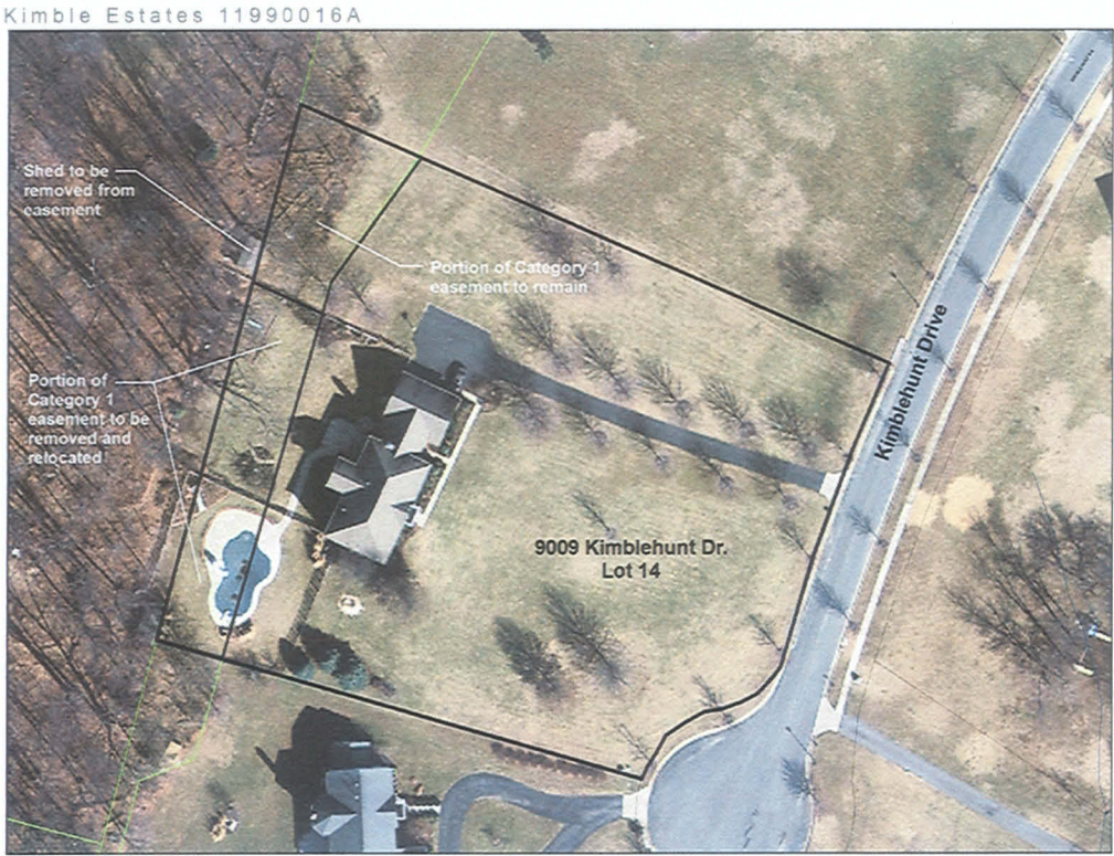
Figure 5: Lot 14 showing portion of easement removed for relocation
