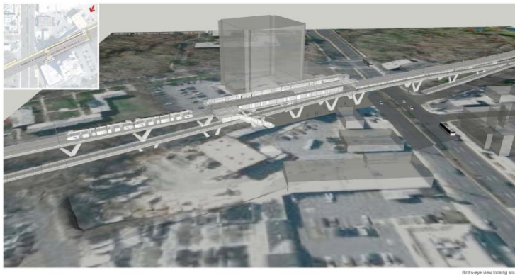
Figure 4: Connecticut Ave Bridge Concept on Piers
