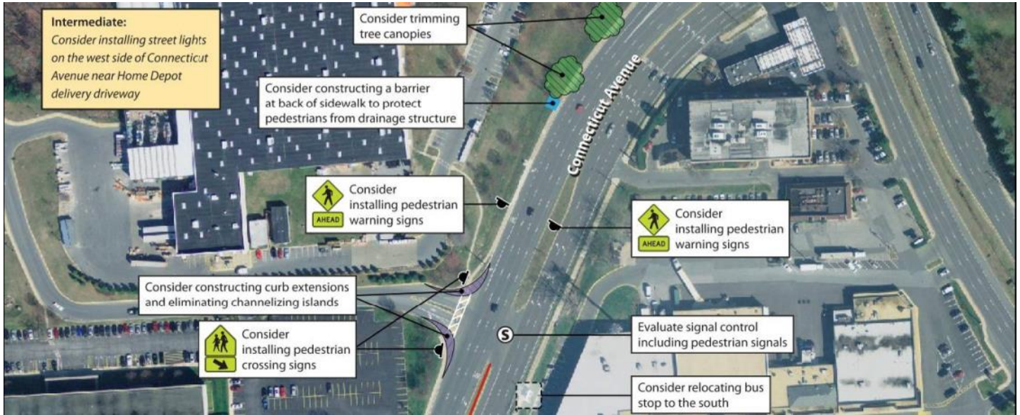
Excerpt from PRSA: Connecticut Ave between Georgia Ave and Aspen Hill Rd Conceptual Improvements
