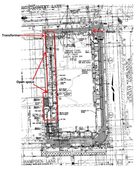
Figure 1 Approved Site Plan with changes indicated by red arrows.
