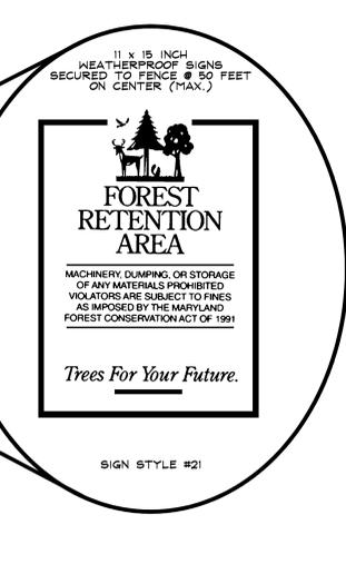
11 x 15 INCH WEATHERPROOF SIGNS SECURED TO FENCE @ 50 FEET ON CENTER (MAX.)
