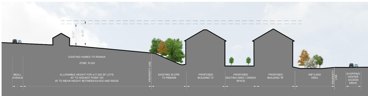
Figure 12: Section thru Buildings A and B showing a drop in elevation, and a buffer of trees between the Subject Property and the adjacent residential properties on Beall Avenue
