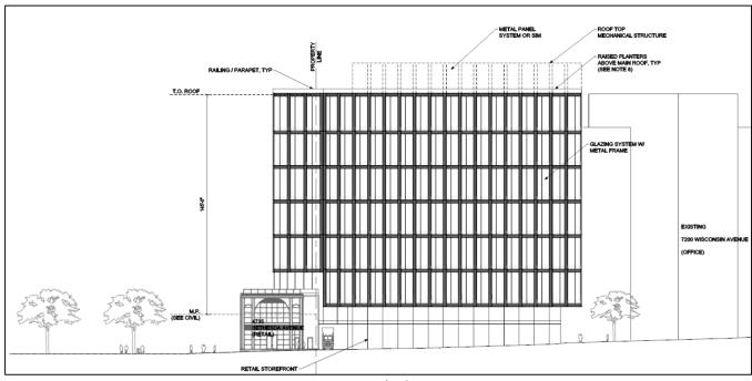
Figure 5-South Elevation
