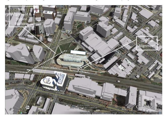
Figure 1 – Purple Line Alignment and Station Location Change at the Silver Spring Transit Center
