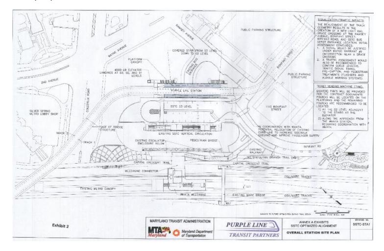
The Purple Line tracks will be located above the 3<sup>rd</sup> level of the SSTC crossing Colesville Road and will descend to a point where is adjacent to the 3<sup>rd</sup> level of the SSTC where Ramsey Street, Bonifant Street and Ripley Street meet. A rendering of the how the new alignment and station location relate to the SSTC and Metrorail / MARC is shown in Figure 8.
