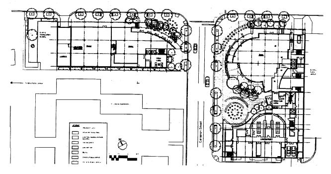
The architectural design for the Project envisions a variety of innovative features including curving glass forms, a seventh floor pedestrian connector, roof gardens connected by a circular stair, arched covered walkways along street level retail shops, geometric roof forms with photovoltaic panels at the proper angular pitch toward sun to generate power as well as artistically designed public spaces. The design embraces the site's role as an urban gateway to Silver Spring.
