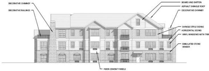
Figure 11: Illustrative design of the west elevation (Fleming Avenue)
