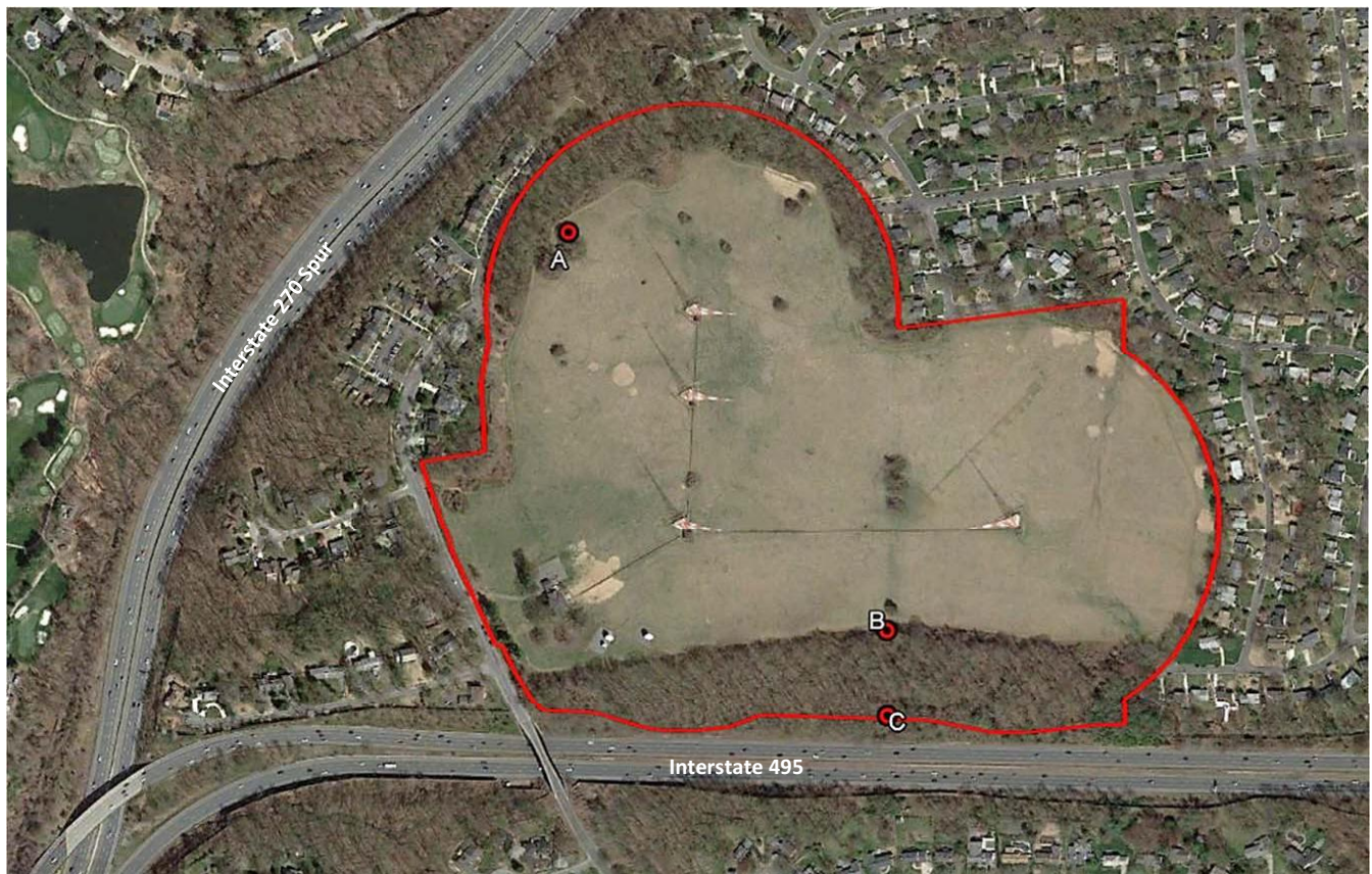
Figure 3: Long-term noise measurement locations.
