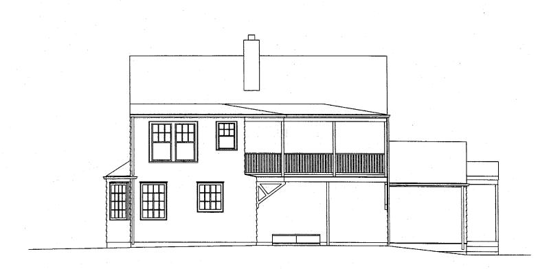
Figure 6. Rear (East) Elevation. The two-storey addition and the bay and the left, as well as the second floor porch are all additions from the late 1930's. Drawing by Jason Gagen, copyright 2004 by Brenneman & Pagenstecher, Inc.
