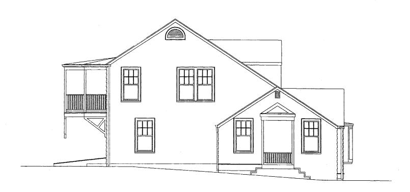
Figure 5. Left (North) Elevation. The projecting bay and portico on the right are part of the 1925 addition. The roofline of the original bungalow was raised in the late 1930's from a 5/12 pitch to an 8/12 pitch to provide more headroom on the second floor. Porch and bump out at left are part of ththe 1930's renovation as well. *Drawing by Jason Gagen, copyright 2004 by Brenneman & Pagenstecher, Inc.*
