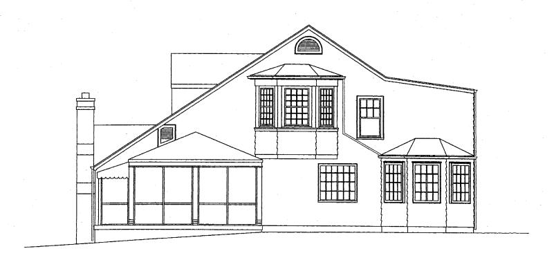
Figure 7. Right (South) Elevation. Both bays are additions from the 1930's. Drawing by Jason Gagen, copyright 2004 by Brenneman & Pagenstecher, Inc.
