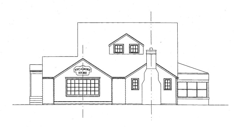
Figure 4. Front (West) Elevation. The two front gables and the porches to either side are all additions from 1925. Note the dormer in the roof of the original bungalow, behind. Drawing by Jason Gagen, copyright 2004 by Brenneman & Pagenstecher, Inc.
